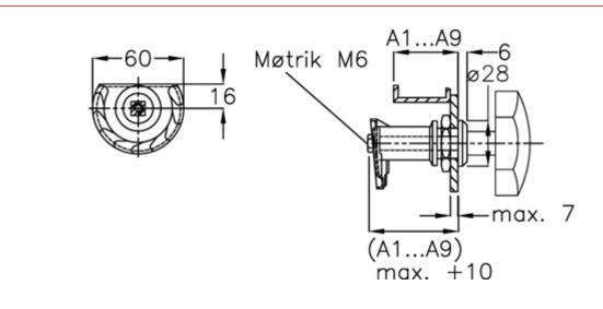
Door + frame thickness = 57-65 Measure type = A9
